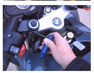
**3.** Loosen the socket head cap screws completely and remove the comfort bars from the fork tubes on one side. Place it on some padding like a towel, on top of the fuel tank to avoid scratches. Clean the surfaces of the fork tubes to remove any dirt, grease and oil.
