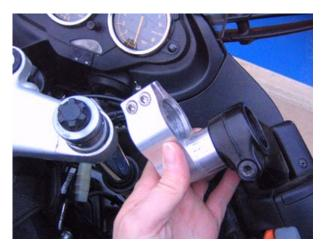
**4.** Turn your forks all the way to the steering lock on the side you are installing for clearance and slack.
