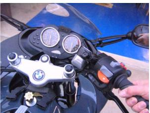
**5.** \*Second! Mount the entire handlebar and barback assembly onto the fork tube. You'll find this is much easier than trying to mount the barbacks first and *then* stretching your wires and cables to get the comfort bars onto the barback's post.
