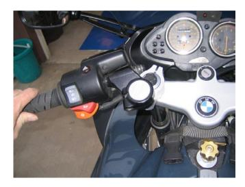
**7. Alignment**: Most people like to align the bar backs parallel and symmetrical, tighten, and then adjust the comfort bars to suit. However, the barbacks have some concentric adjustment on the fork tube. Use your own discretion and adjust the set-up to fit your ergos best. Adjust the barbacks and comfort bars to clear the fuel tank at full steering lock in both directions.
